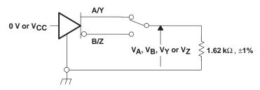
Figure 7. Maximum Steady State Output Voltage
