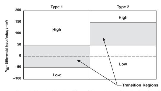
Figure 28. Expanded Graph of Receiver Differential Input Voltage Showing Transition Region
