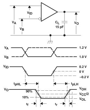
NOTES:A. All input pulses are supplied by a generator having the following characteristics: t<sub>r</sub> or t<sub>f</sub> ≤ 1 ns, frequency = 50 MHz, duty cycle = 50 ± 5%. C<sub>L</sub> is a combination of a 20%-tolerance, low-loss ceramic, surface-mount capacitor and fixture capacitance within 2 cm of the D.U.T. B. The measurement is made on test equipment with a –3 dB bandwidth of at least 1 GHz.
