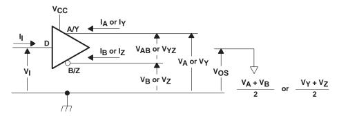
Figure 1. Driver Voltage and Current Definitions
