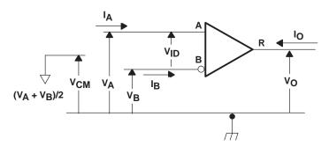
Figure 9. Receiver Voltage and Current Definitions
