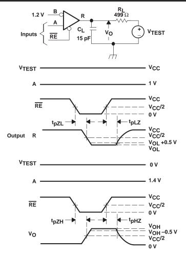
NOTES:A. All input pulses are supplied by a generator having the following characteristics:  $t_{\Gamma}$  or  $t_{f} \le 1$  ns, frequency = 500 kHz, duty cycle =  $50 \pm 5\%$ .
