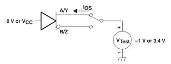
Figure 4. Driver Short-Circuit Test Circuit
