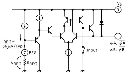
$V_{REG}$  output voltage can be selected with  $R_{REG}$  exterior resistance.
