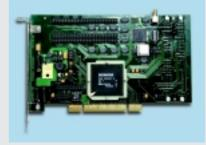
The EASY256/3456 is a PCI based evaluation board. Together with the low level software driver, this complete evaluation kit is speeding-up your development process.
